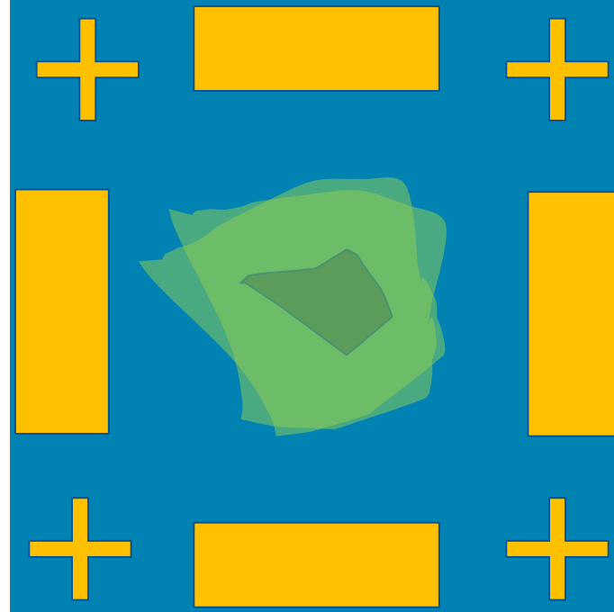
E-beam litho: Align mark, bonding pads Ti 10/Au 60/ Pd 20nm
